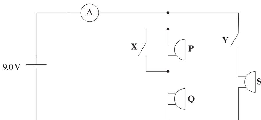
In the above circuit, buzzers **P**, **Q** and **S** are controlled using switches **X** and **Y**. **The buzzers are identical and their resistances remain constant.**
